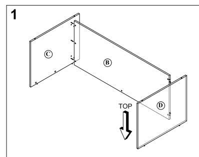
Turn Top Panel (A) upside down and insert Cam Lock pins (1) into top panel and into side panels (C,D). Insert Klix Cams (2) in Side Panels (C,D) and back panel (B). Attach Back Panel (B) to side panels (C,D) and Top Panel (A). Turn Klix Cam to tighten.
